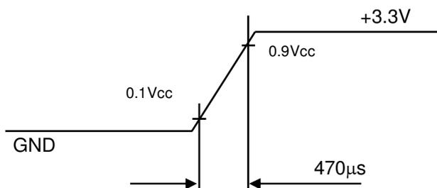
Note (3) The specified power supply current is under the conditions at  $V_{cc} = 3.3\text{ V}$ ,  $T_a = 25 \pm 2\text{ }^\circ\text{C}$ ,  $f_v = 60\text{ Hz}$ , whereas a power dissipation check pattern below is displayed.
